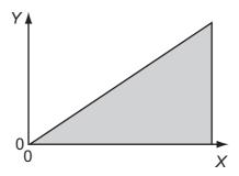
The shaded area represents the total strain energy stored in stretching the wire.
