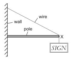
The force exerted by the pole at point X is F, and the tension in the wire is 40 N.
