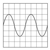
The setting of the time base is then changed from  $10\,\mathrm{ms\,cm^{-1}}$  to  $20\,\mathrm{ms\,cm^{-1}}$  and the Y-sensitivity is unaltered.
